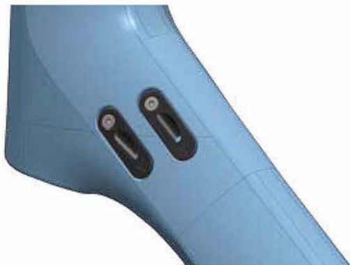
2.3mm Hole and Cable Stop for Mechanical Derailleur Cables
